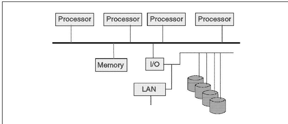
Figure 11. A Typical SMP Configuration
