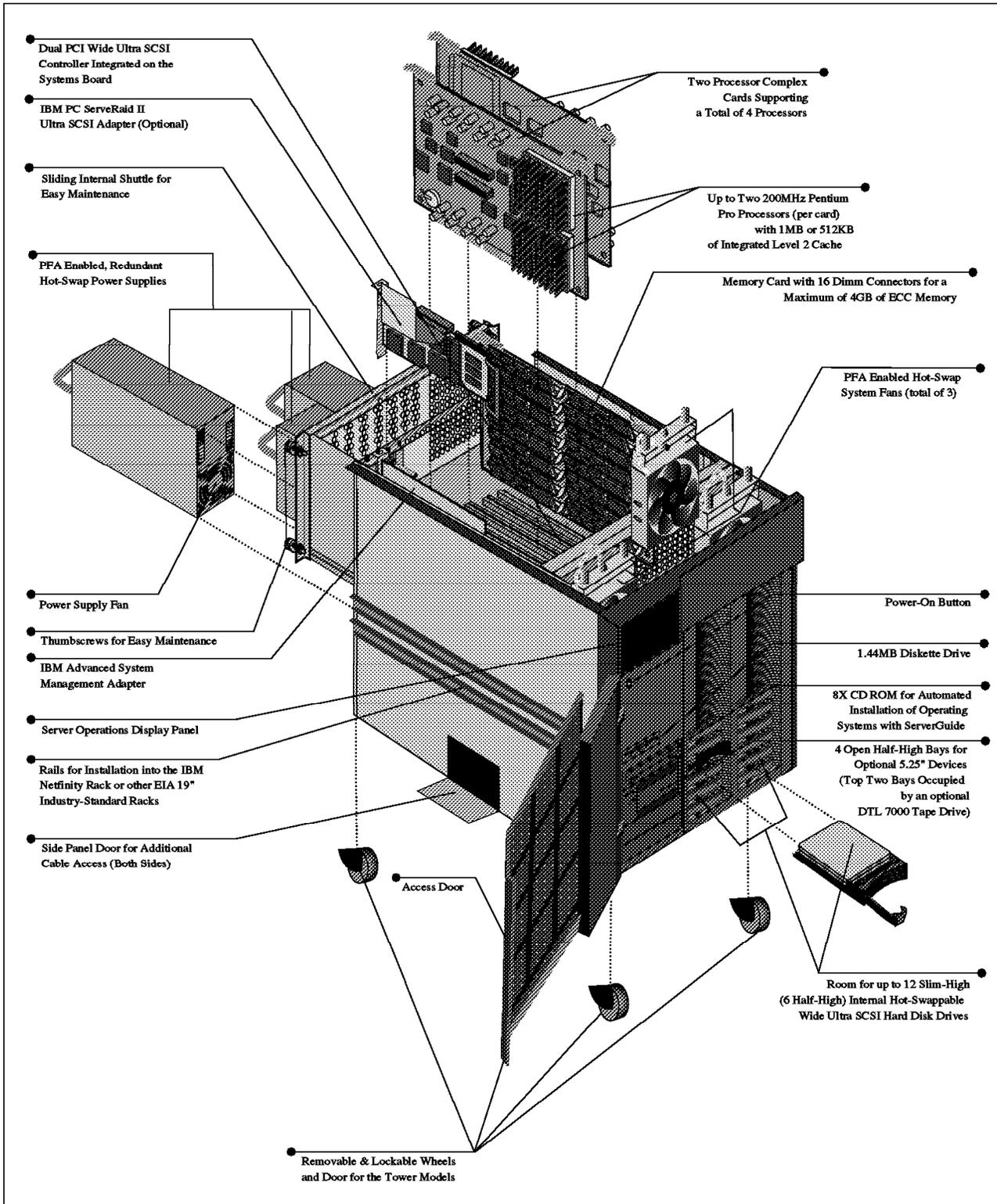
Figure 58. Exploded View of the Netfinity 7000
