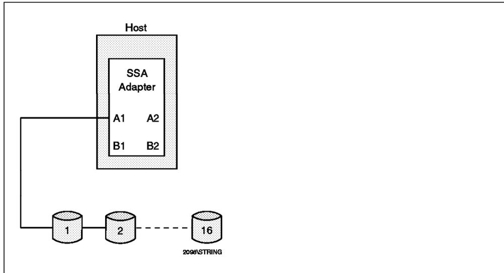
Figure 30. A String. A string has only one cable to the host adapter. If this cable were to fail, all communication with the disks would be lost. For this reason a string configuration is not recommended.
