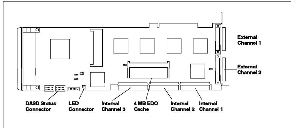
Figure 73. The IBM ServeRAID II Ultra SCSI Adapter
