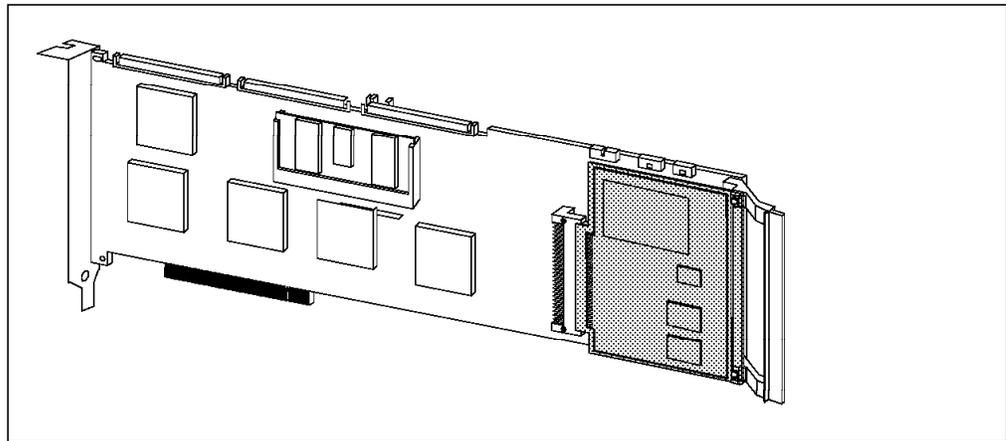
Figure 75. IBM ServeRAID II Ultra SCSI Adapter with 8 MB Battery-Backup Cache Installed (Shown in Gray)
