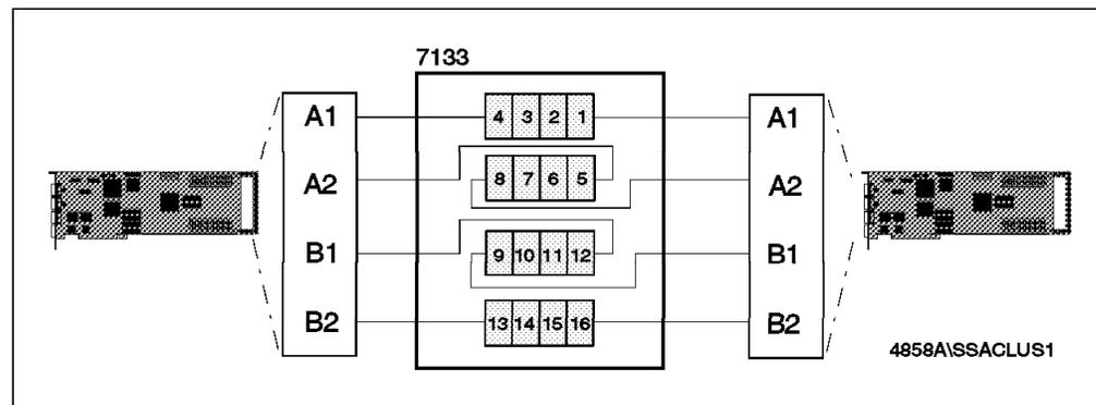
Figure 77. SSA RAID Cluster Configuration. The two SSA RAID Cluster Adapters are connected to one (or more) 7133s such that if one server fails, the other server can take over all disks.
