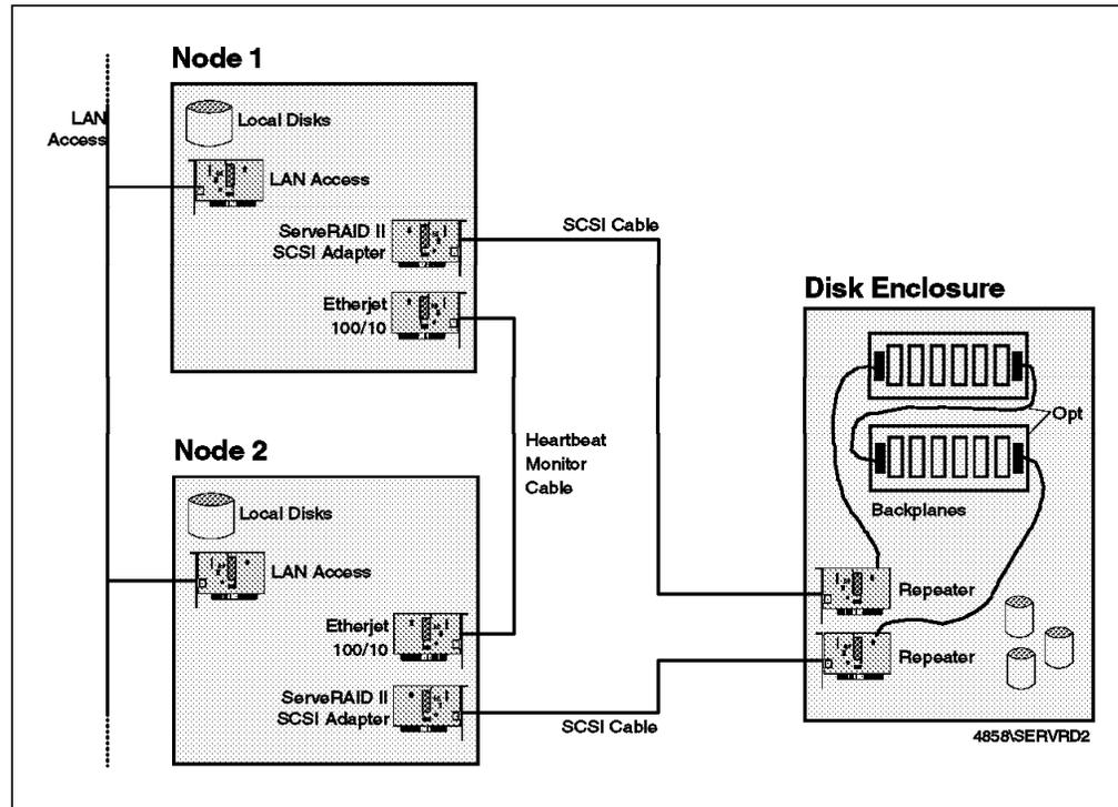
Figure 25. Connecting Two SCSI Host Adapters to One SCSI Bus. This configuration is used with VHA for OS/2 and IntranetWare.
