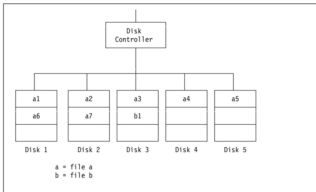
Figure 32. RAID-0 (Block Interleave Data Striping without Parity)
