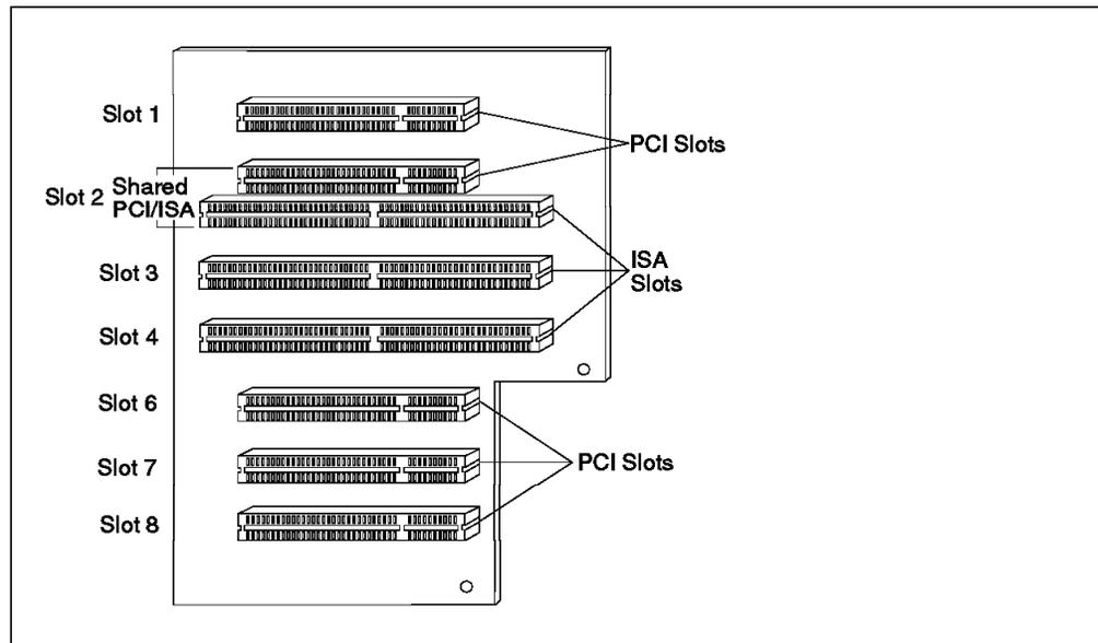
Figure 44. IBM PC Server 315 - Riser Card
