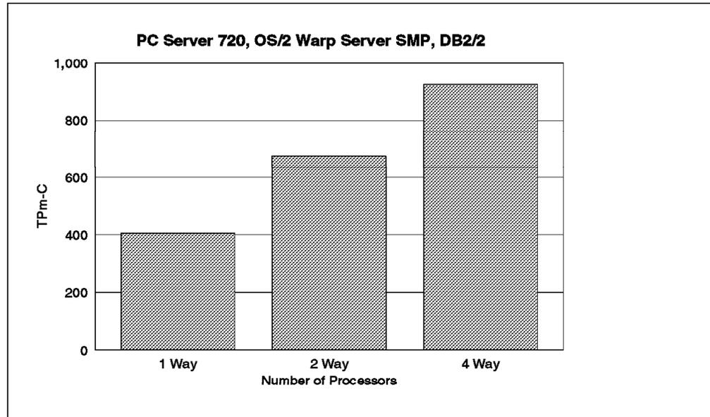
Figure 2. Comparing Transactions per Minute for Multiple Processors
