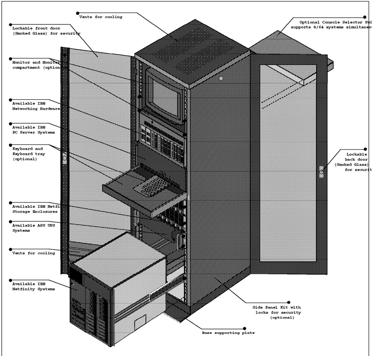
Figure 60. Exploded View of the IBM Netfinity Rack Enclosure
