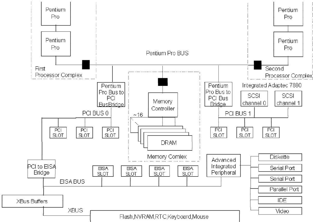
Figure 14. PCI Configuration in the PC Server 704
