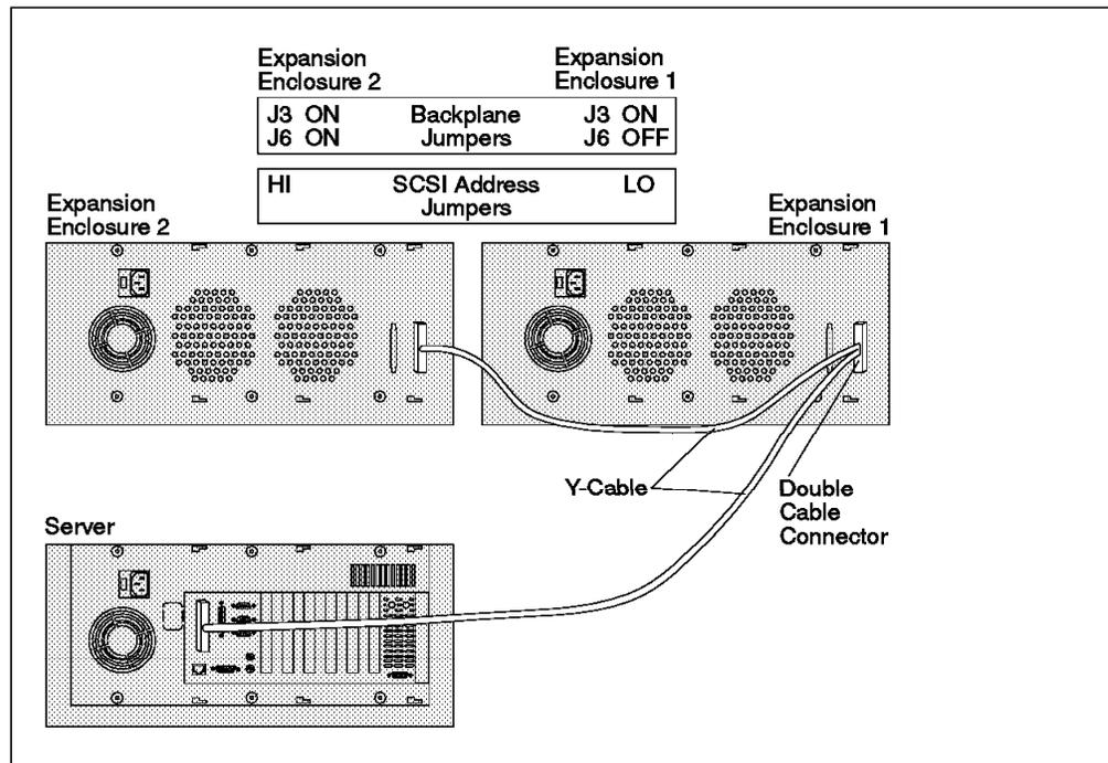
Figure 65. Daisy Chaining Two 3519s Together. The 3519s are connected together using the Storage Extender Cable (#94G7594).
