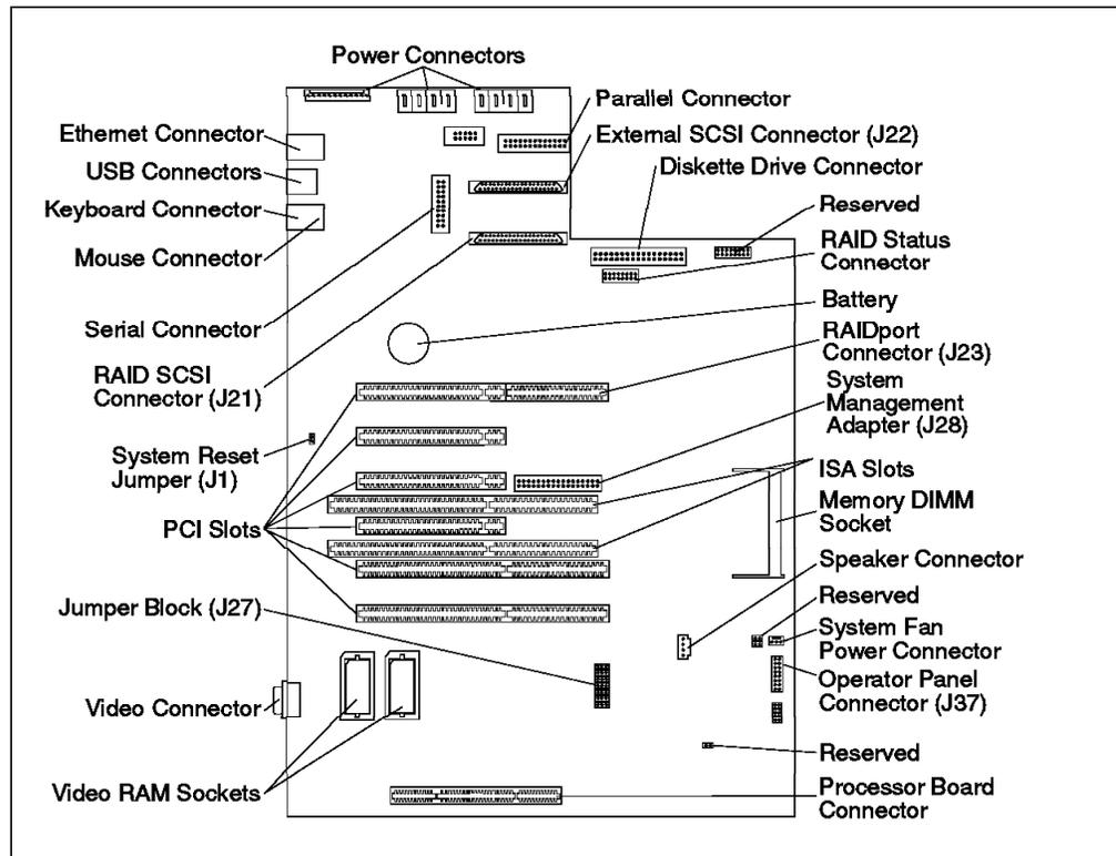
Figure 52. View of the IBM PC Server 330 System Board
