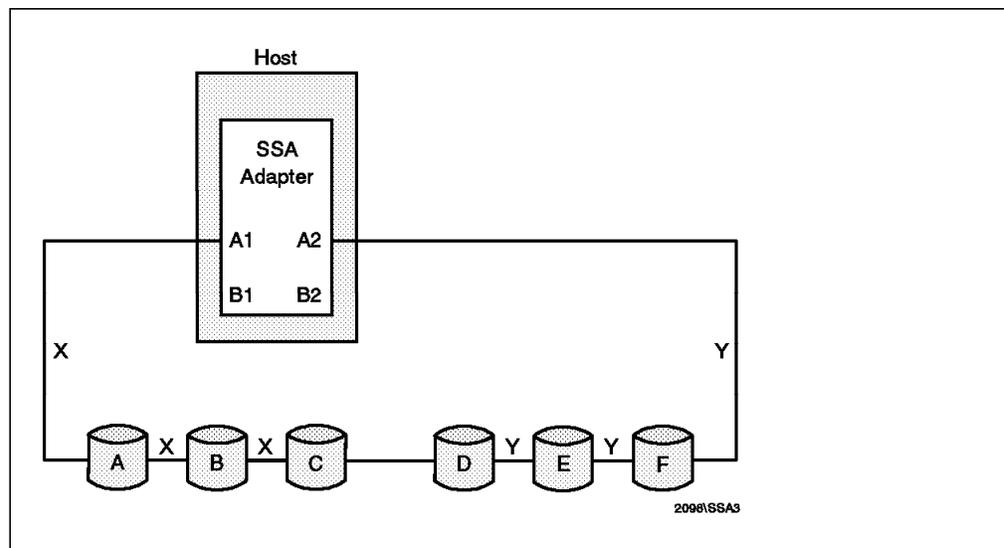
Figure 31. An Example of SSA Spatial Reuse. The single host adapter can transmit data X to or from drives A, B and C at the same time as it is transmitting data Y to or from drives D, E and F.
