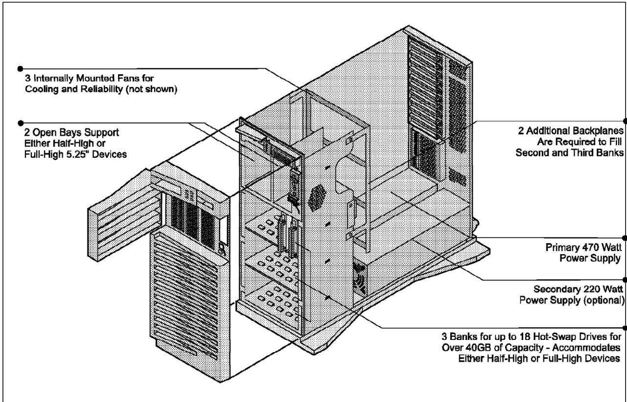
Figure 63. Exploded View of the IBM 3518 PC Server Enterprise Expansion Enclosure
