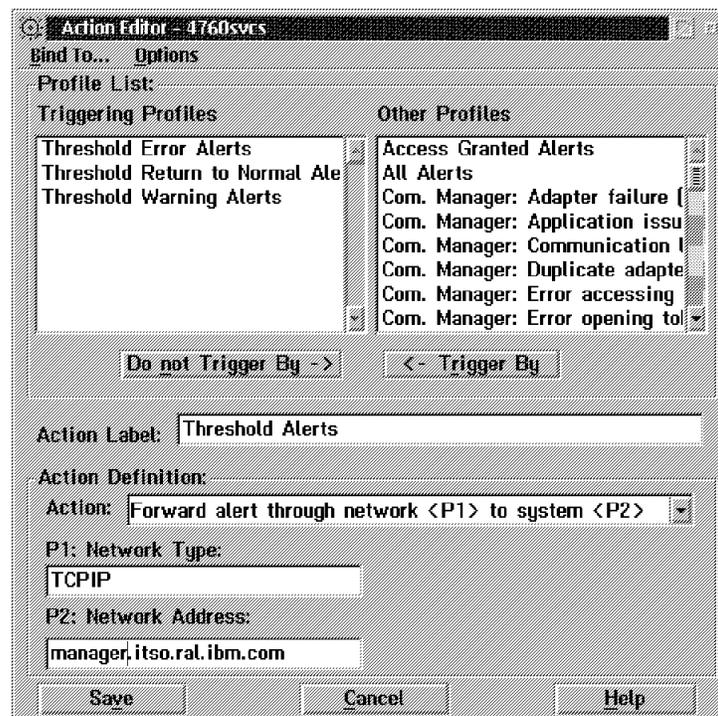
Figure 101. Defining an Alert if CPU Threshold is Reached.
