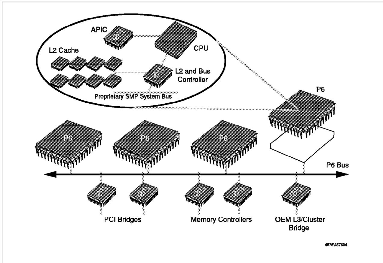
Figure 7. The Pentium Pro in a Four-Way SMP Configuration
