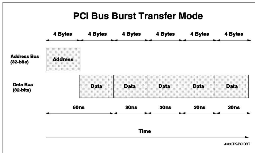
Figure 12. PCI Bus Burst Transfer at 33 MHz
