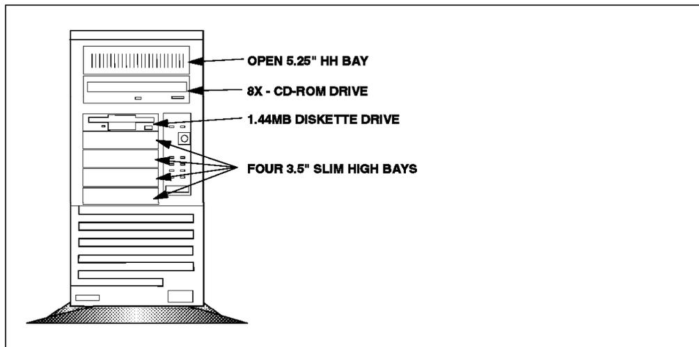
Figure 48. IBM PC Server 325 Expansion Bays
