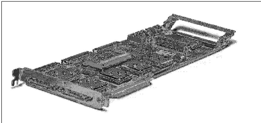
Figure 72. The IBM ServeRAID II Ultra SCSI Adapter
