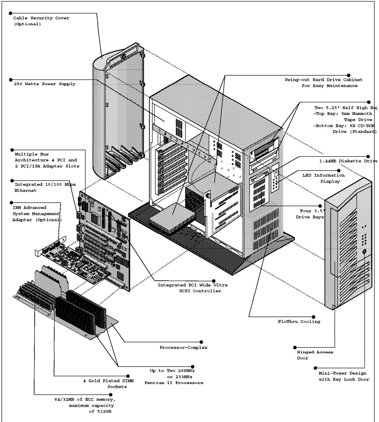
Figure 45. Exploded View of the IBM PC Server 325 Mini-Tower Model
