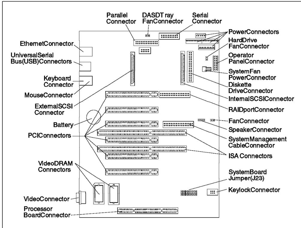
Figure 47. IBM PC Server 325 System Board
