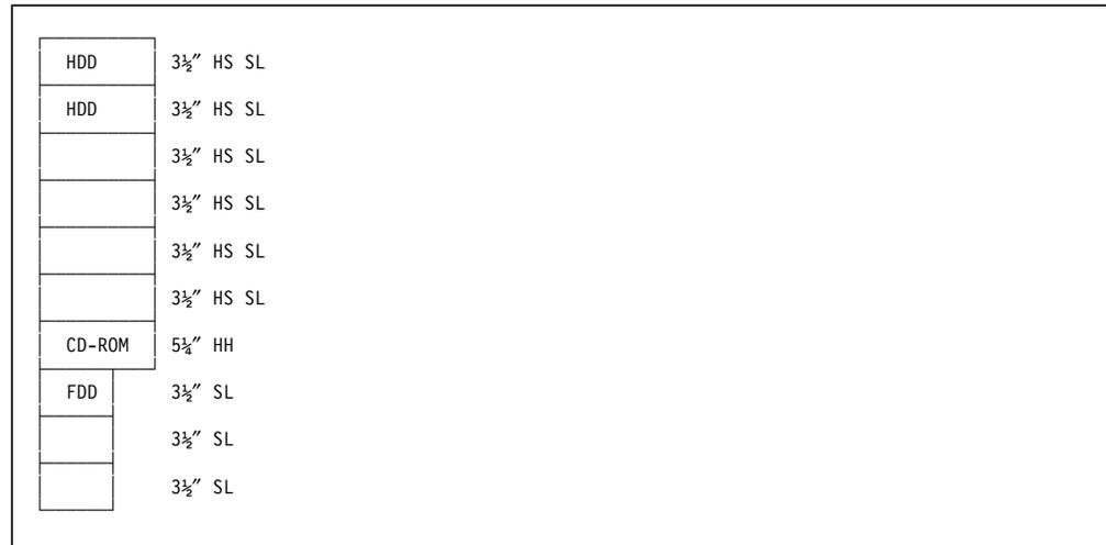
Figure 53. Server 330 Expansion Bays. (HH = half-high; HS = hot-swap; SL = slimline)
