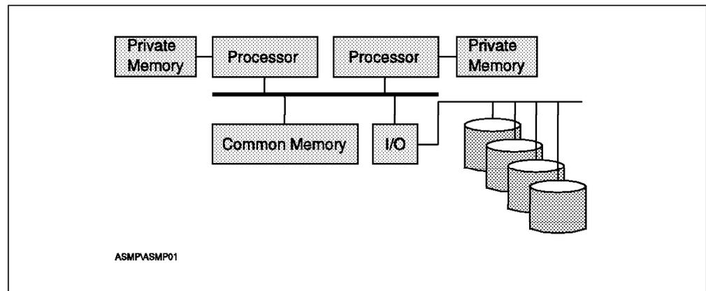
Figure 9. Asymmetric Multiprocessing Example 1. This configuration has multiple memory units with some of those not shared by all processors.
