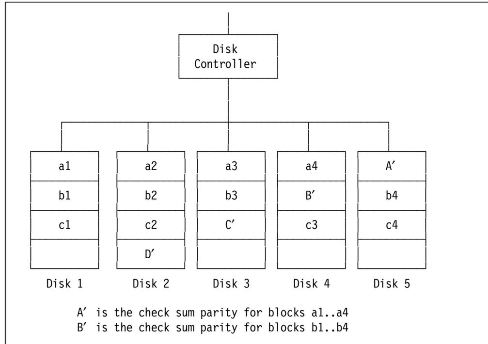
Figure 35. RAID-5 (Block Interleave Data Striping with Skewed Parity)
