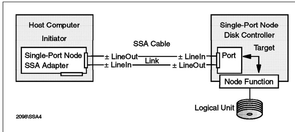
Figure 28. SSA Link - A Closer View
