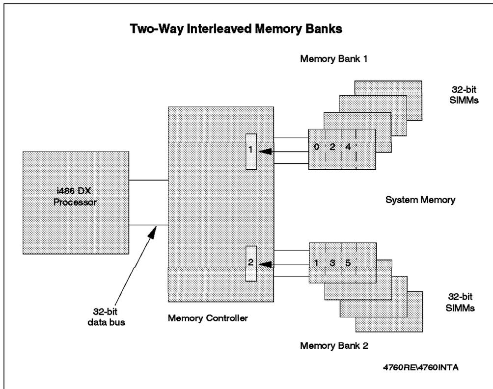
Figure 21. i486-Based Two-Way Interleaved Memory System
