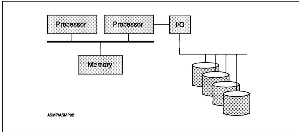
Figure 10. Asymmetric Multiprocessing Example 2. This configuration has one processor doing all I/O.
