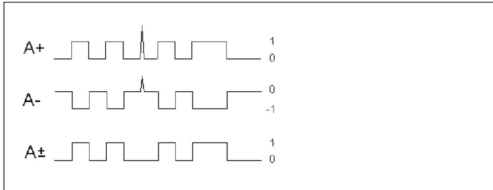
Figure 24. SCSI Differential Example
