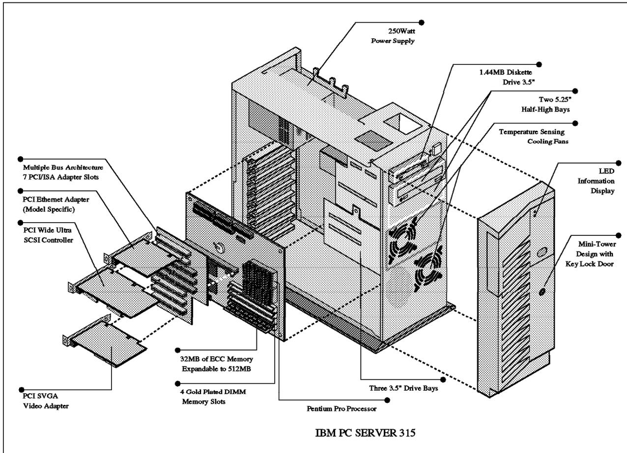
Figure 43. Exploded View of the IBM PC Server 315
