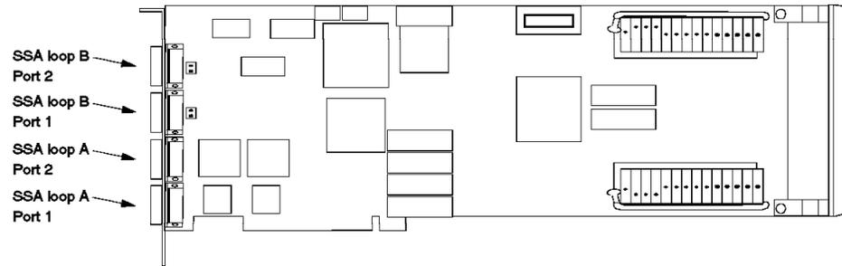
Figure 76. SSA RAID Cluster Adapter
