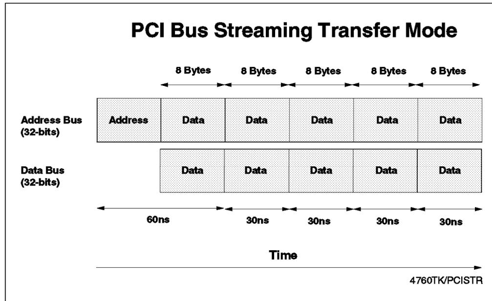
Figure 13. PCI Bus Streaming Mode at 33 MHz
