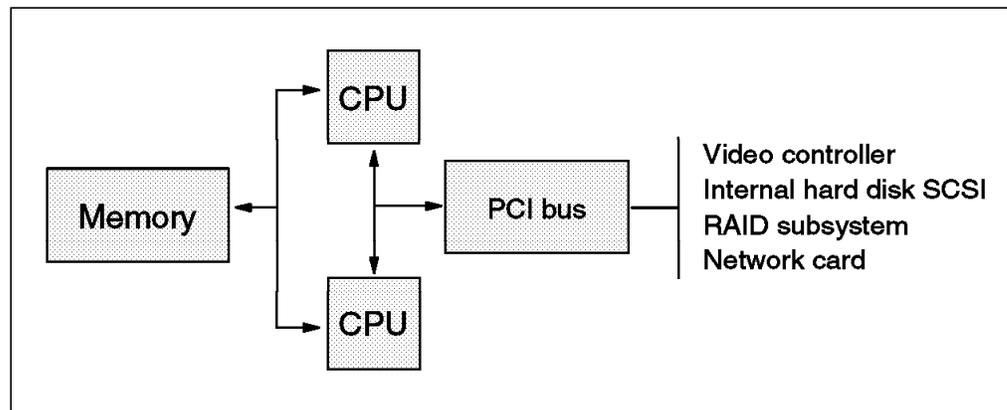
Figure 15. System Without I·O Architecture
