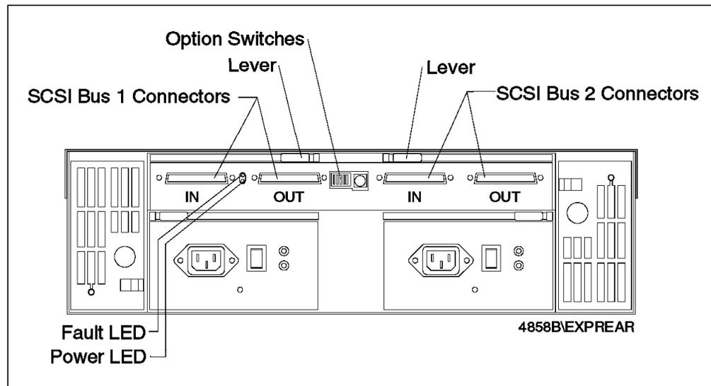
Figure 68. Netfinity EXP10 Rear Controls, Indicators and Connectors
