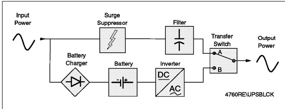
Figure 37. UPS Block Diagram
