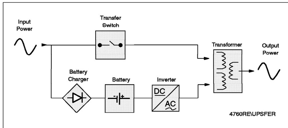
Figure 40. The Standby-Ferro UPS
