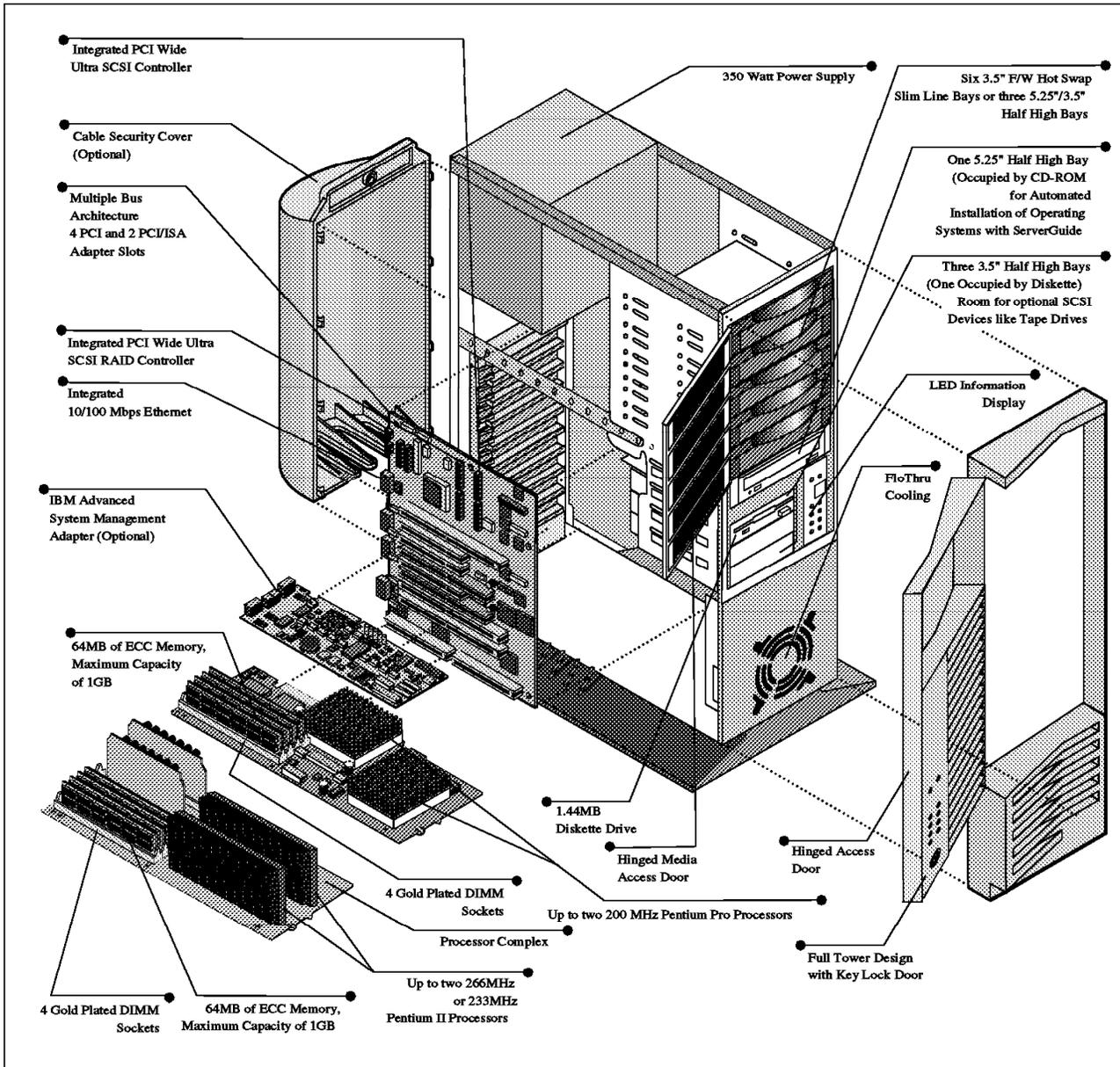
Figure 49. Exploded View of the IBM PC Server 330
