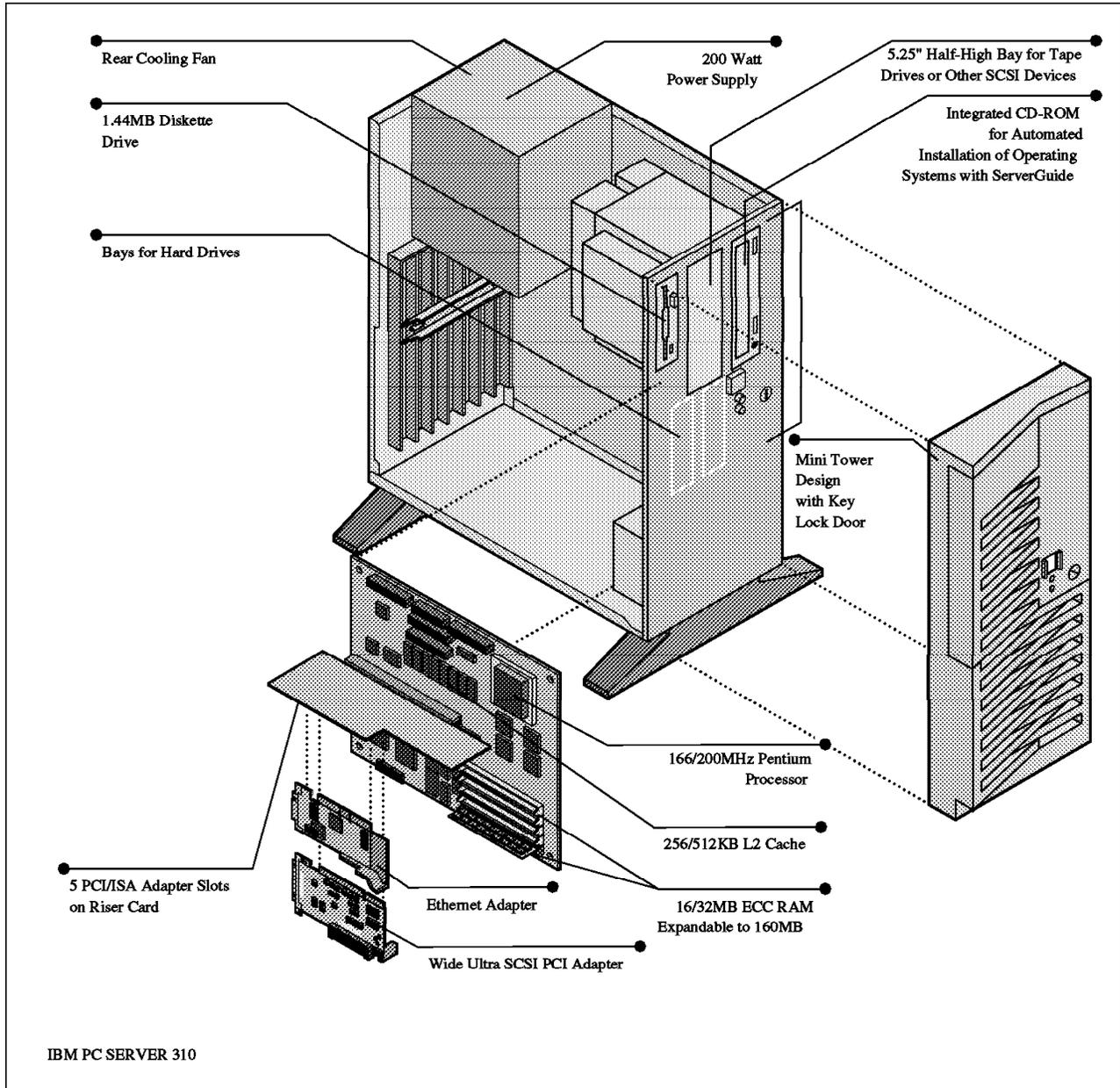
Figure 42. Exploded View of the IBM PC Server 310
