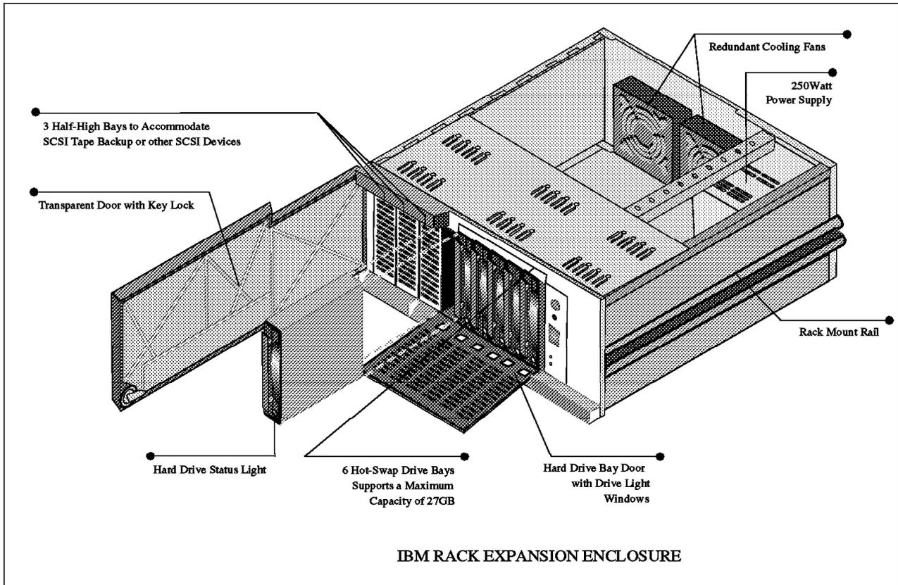
Figure 64. Exploded View of the IBM 3519 Rack Storage Expansion Enclosure
