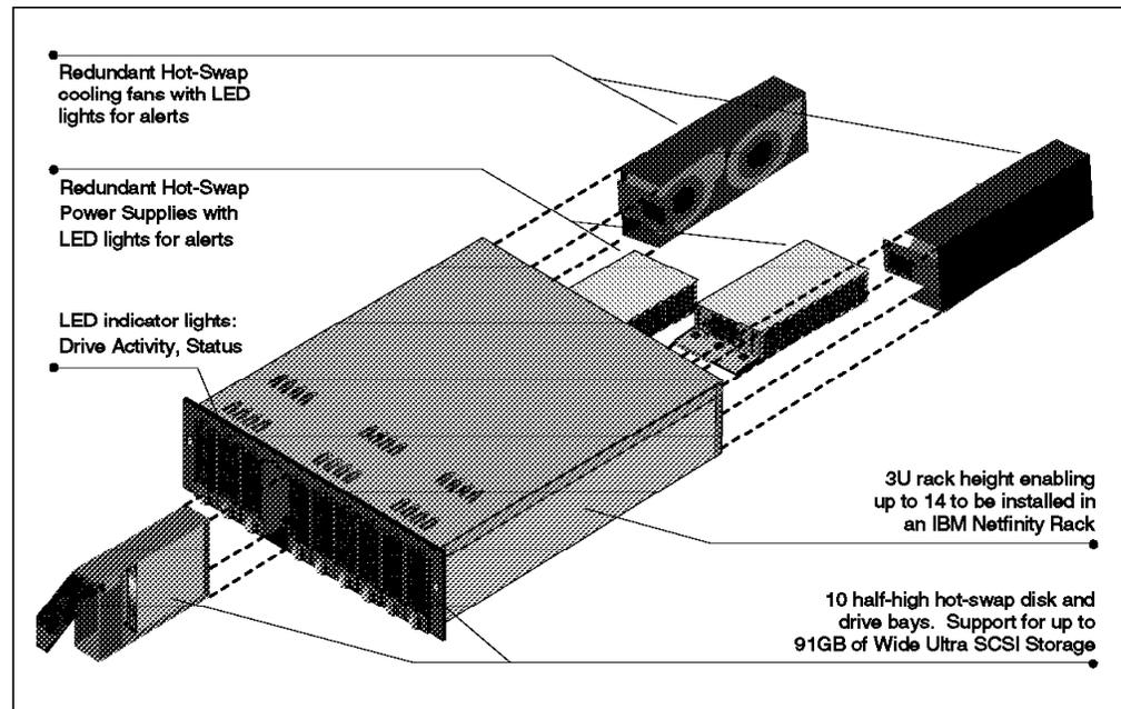
Figure 66. Exploded View of the IBM Netfinity EXP10
