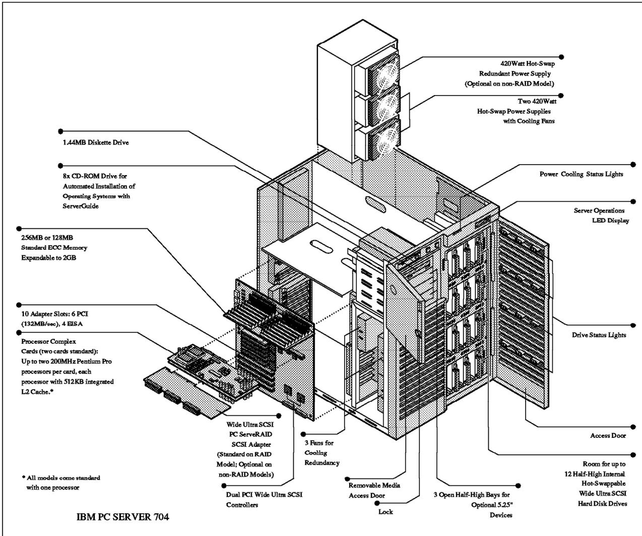
Figure 56. Exploded View of the Server 704 200 MHz
