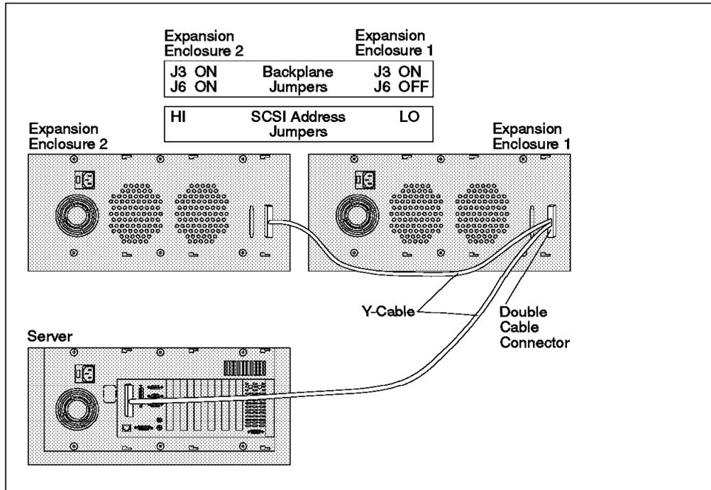
Figure 26. Daisy Chaining Two 3519s Using a SCSI Repeater. The 3519s are connected together using the Storage Extender Cable (#94G7594).
