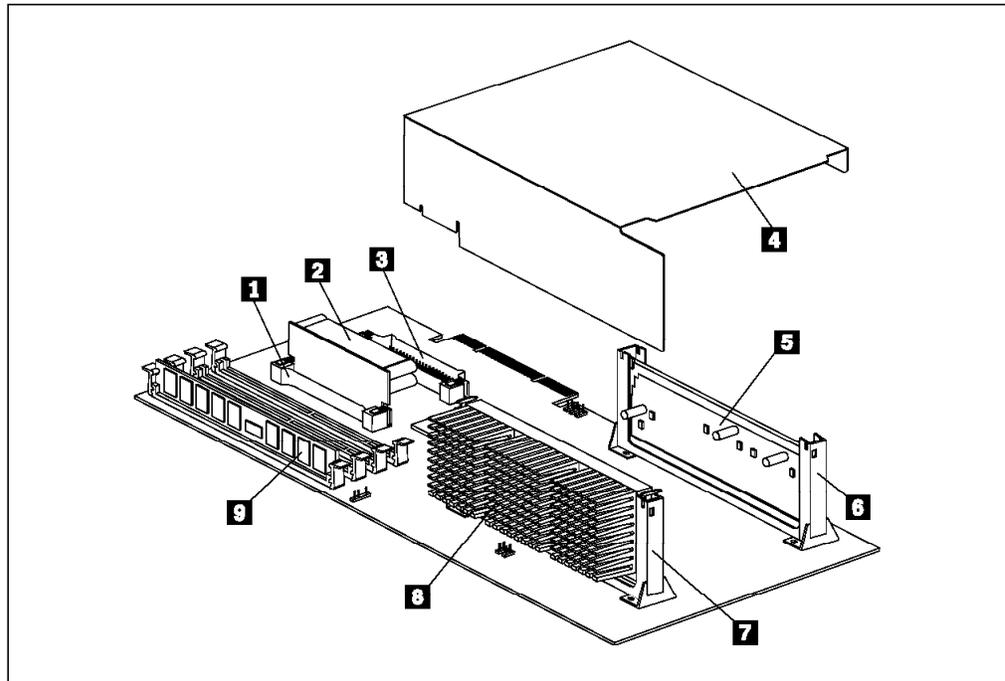
Figure 46. IBM PC Server 325 Processor Board
