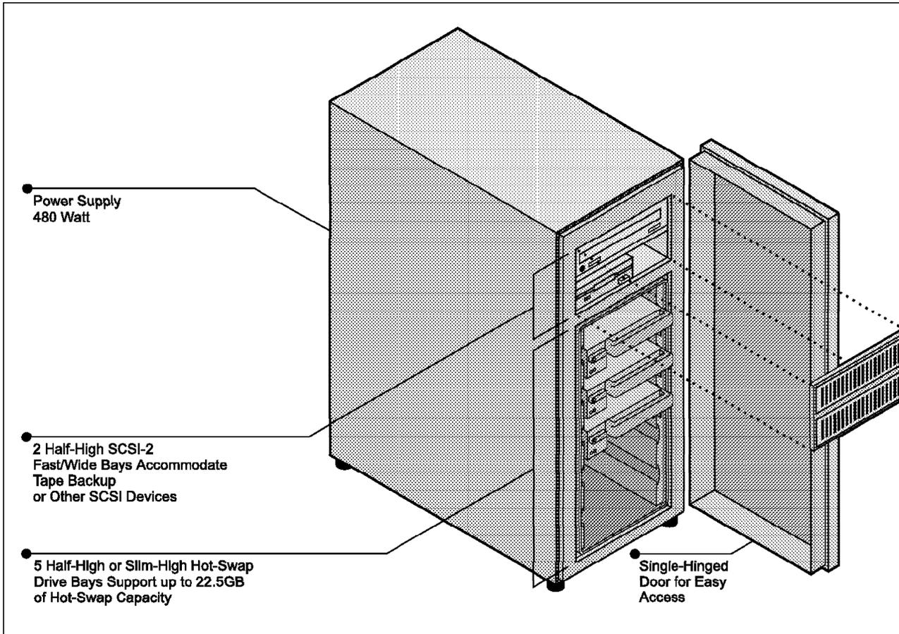
Figure 62. Exploded View of the IBM 3517 SCSI Multi-Storage Enclosure
