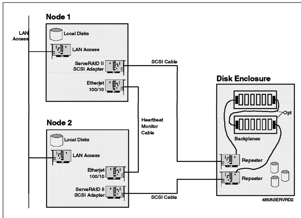
Figure 69. Repeater Connectivity. Two servers connected to a shared external enclosure using two Enhanced Repeaters.
